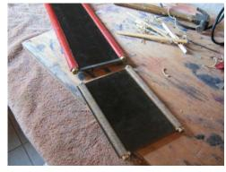
7. Here's the shortened reed. I plan to use the leftover piece in my tension box during sectional warping.
