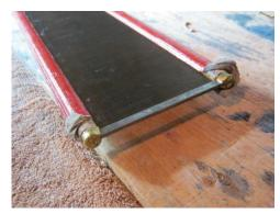
6. The bar is slid back into the groove, the brass caps replaced and nailed in. Finally, the tape is re-adhered until it's even with the brass caps and the excess is trimmed.
